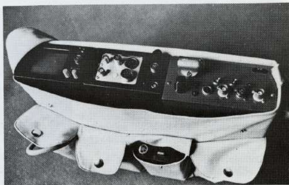
Canvas bag containing UHF receiver (FRX 800), monitor (KWA 52) and video insert system (INS 26).
